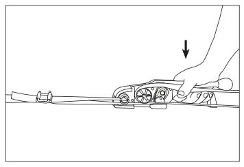
4 Push lever down to cut tail and open gripper foot. Hold lever in downward position and rotate tool to the side to remove tool from strap.
