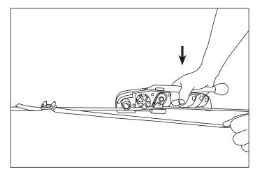
Position tool approximately 12 inches away from buckle. Hold lever in downward position to open gripper foot. Place strap under cutter, under drum and under gripper foot. Release lever to clamp gripper foot down onto strap.
