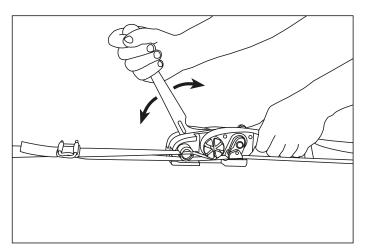
3 Crank lever back and forth to tension strap. Tensioning is complete when top leg of buckle closes down and touches base of buckle.
